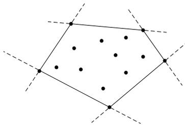
Figure 2. Pivoting an infinite large disk around the point set yields the convex hull.
