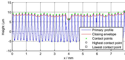
Figure 3. The extracted envelope profile with contact points (rolling element 5mm radius).
