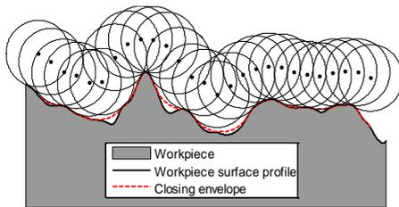
Figure 1. Closing envelope obtained by rolling a disk over the profile.
