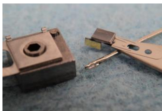
Figure 2: Plasmonic writing head with mirror in place for measurement.
