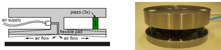
Fig. 1. Active aerostatic bearing (a) sketch and working principle (b) prototype
