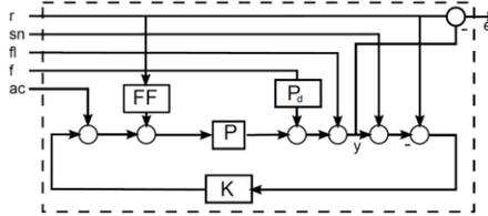
Fig. 2. Closed loop control system with main disturbances
