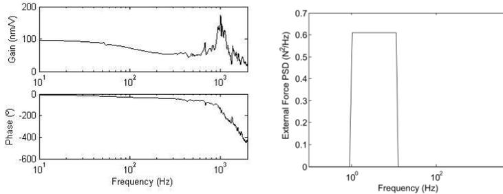
Fig. 3. (a) FRF of active bearing plant  $P$  (b) PSD of applied external force  $f$
