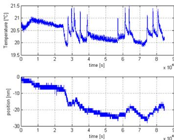
Figure 5: Reading head stability results
