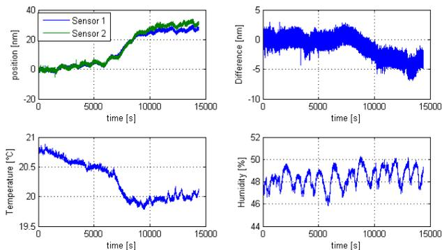
Figure 3: Drift comparison between two capacitance sensor weather stations.
