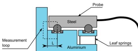
Figure 2: Capacitance probe mounting in weather station.
