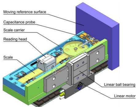
Figure 1: Test setup of the moving scale measurement system
