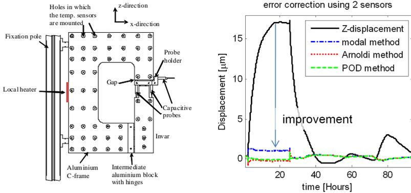
Figure 1 *left*) Mirror mechanism with a spider *right*) Measured z-displacement and the improvement using 2 temperature sensors and a correction based on 2 thermal-mode-shapes, 2 Arnoldi projection shapes and 2 POD-based projection shapes.
