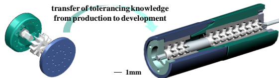
Figure 2: Feedback of manufacturing data from previously designed project (left) eased tolerancing of currently developed system “micro gas turbine” (right)
