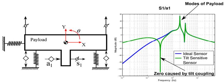
Figure 3: A typical layout of a vibration isolation system (left). The horizontal actuator ( $a_1$ ) and sensor ( $s_1$ ) suffer from tilt horizontal coupling. Open-loop Bode diagram of a sky-hook control loop showing the difference between an ideal sensor and a sensor suffering from tilt coupling (right).
