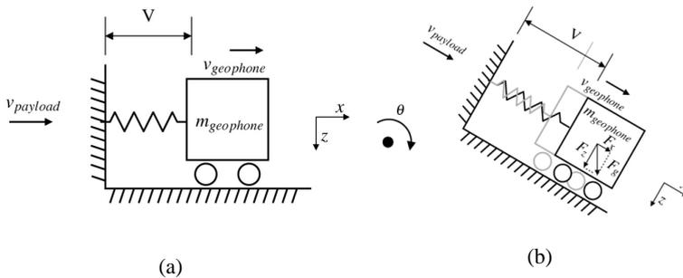
Figure 2: Horizontal geophone. The difference in velocity between the payload and the mass of the geophone is a measure for the relative velocity of the payload. A voltage,  $V$  is induced by a relative displacement of a magnetic field and a coil (a). The geophone is measures tilt through the influence of gravity forces  $F_g$ . (b)
