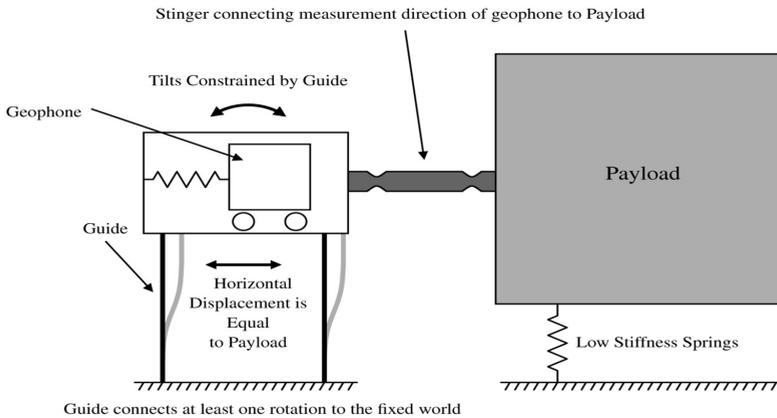
Figure 4: Novel idea for solving issues regarding tilt horizontal coupling. The Guide stiffness allows a horizontal motion of the geophone, while constraining tilting motions. In the measurement direction the geophone is stiffly connected to the payload.
