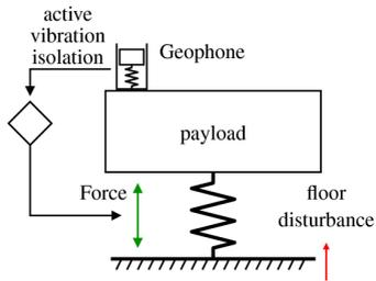
Figure 1: Vibration isolation using sky-hook damping. The geophone forms an absolute velocity signal passed through a controller generating a damping force.
