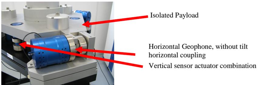
Figure 5: AVI vibration isolation platform with novel horizontal sensors without tilt horizontal coupling
