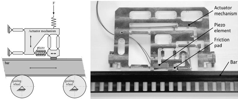
Figure 2: Concept and realisation of CSU piezo actuator
