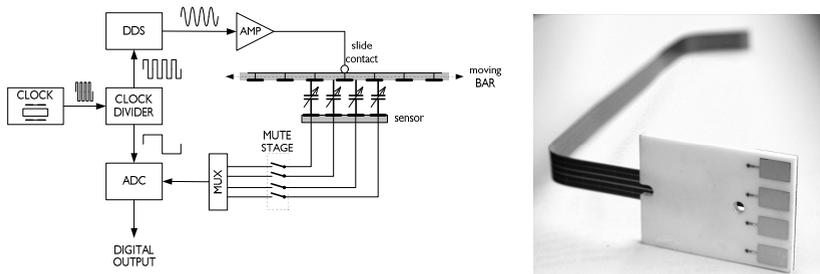
Figure 3: CSU measurement scheme and sensor
