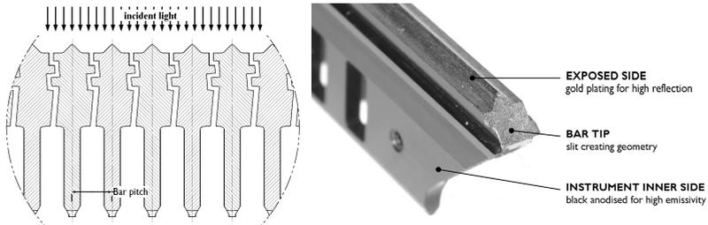
Figure 3: Concept and realisation of CSU bar
