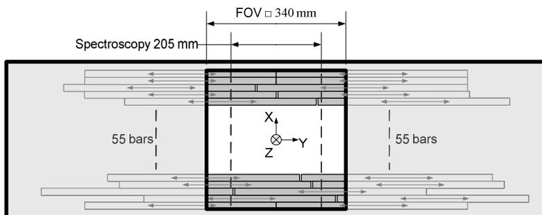
Figure 1: Concept layout of the configurable slit unit
