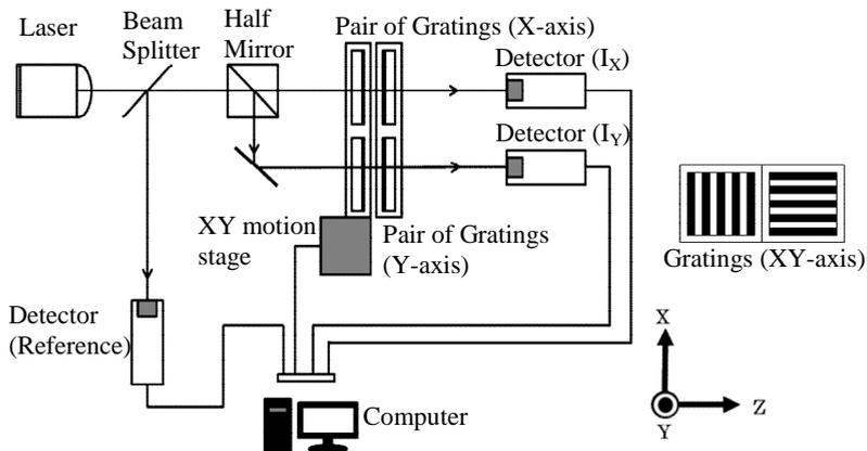
Figure 1: Schematic diagram of the proposed biaxial position sensor
