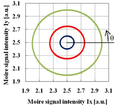
Figure 3: Results of circular interpolation position automatic control
