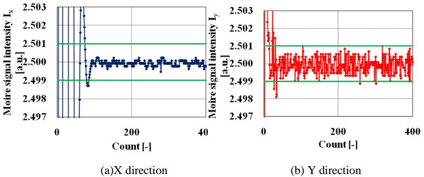
Figure 2: Results of point to point automatic control for (a)X and (b)Y directions
