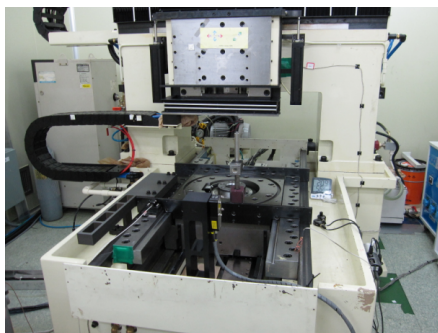
Figure 1. The 4-axis machine tool which is adopting hydrostatic bearings.
