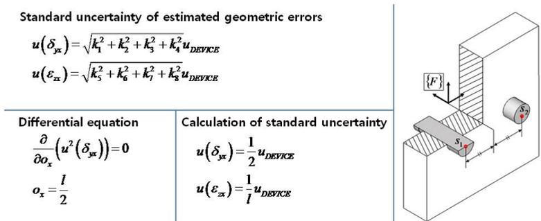
Figure 3: Proposed positions of reference coordinate and sensors
