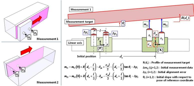
Figure 1: Measurement principle of novel reversal method
