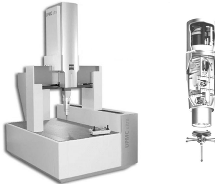
Figure 1: UPMC Ultra CMM with active scanning system (schematic right)
