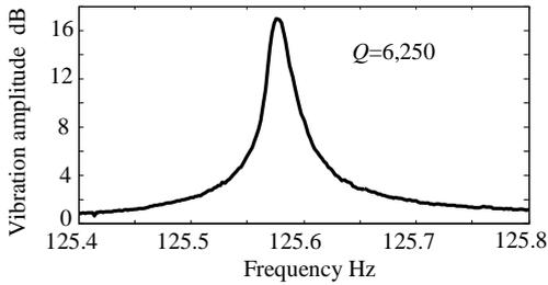
Figure 2: The tuning fork resonance
