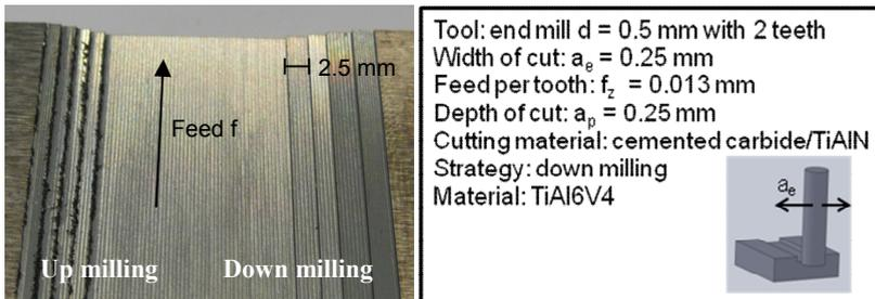
Figure 2: Burr formation when milling TiAl6V4 with 0.5 mm diameter end mill
