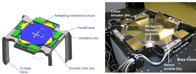
Figure 1 Drive and control concept using air bearings, linear motors, linear encoders and a force frame
