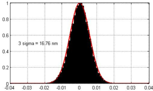
Figure 2. Repeatability error distribution for 1350 small moves,  $3\sigma$  value = 16.76 nanometer (measurement error of 1 nanometer included)
