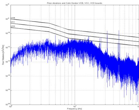
Figure 3. Disturbances from floor vibrations measured by geophones as a function of frequency. Floor is at VC-C specification if we neglect peaks at 48 and 32 Hz due to one single disturbance source.
