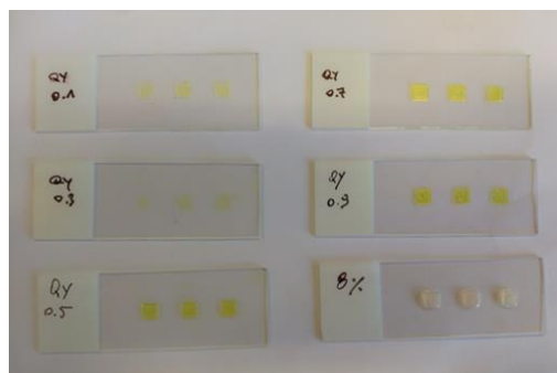
Figure 2. AUP samples cured with the light-box set-up. Increasing concentrations of photo-absorber results in visually thinner films.
