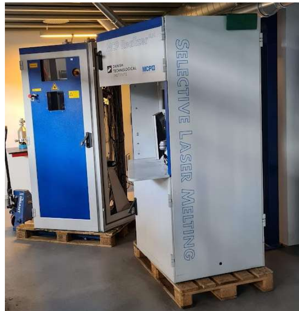
Figure 2. Legacy LPBF system, Realizer 250
