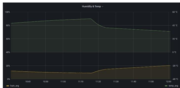
Figure 4. Dashboard with the humidity and temperature reading of the build chamber.
