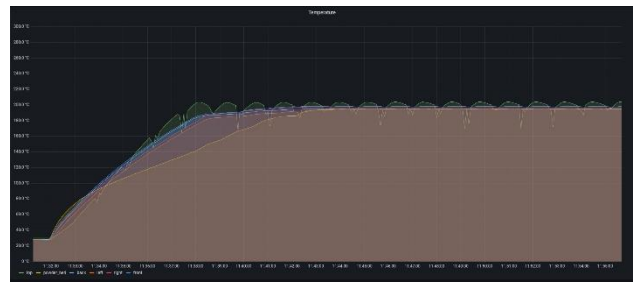
Figure 2. Dashboard with the temperature readings during the powder bed heating up.
