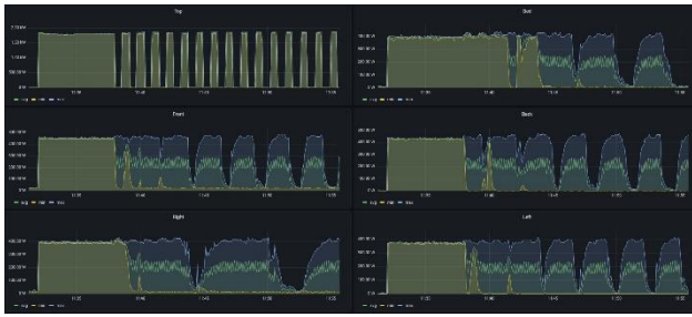
Figure 5. Dashboard with the power consumption during the powder bed heating up.
