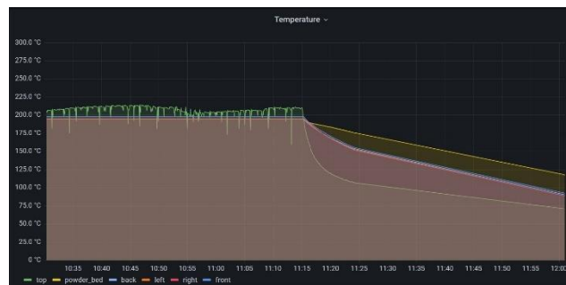
Figure 3. Dashboard view with the temperature readings during a cooldown process.
