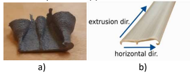
Figure 2. a) CF-PEEK die replica; b) extrudate of ABS
