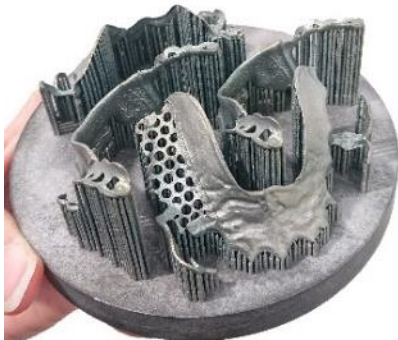
Figure 1 Removable Partial Dentures on the build platform after printing
