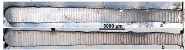
Figure 7. Etching of samples a) without control, b) with OCT control (NaOH etching). Cutting plane perpendicular to the feed direction
