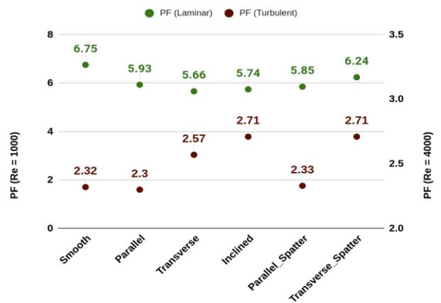
Figure 8. Performance Factor ( $PF$ ) x 100 for various channels for the laminar and turbulent flow cases considered.
