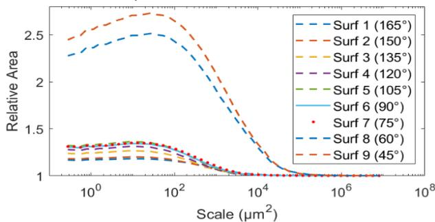
Figure 1. Relative Area analysis of AM different surfaces [5].
