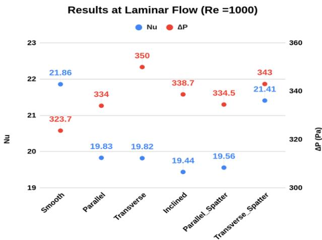
Figure 6. Nusselt Number ( $Nu$ ) and Pressure Drop ( $\Delta P$ ) for various channels for the laminar flow case.
