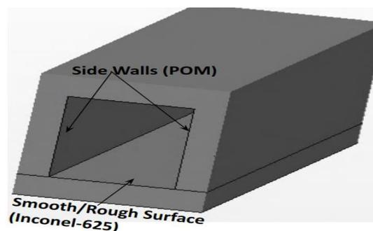
Figure 3. CFD Model with artificial AM surfaces
