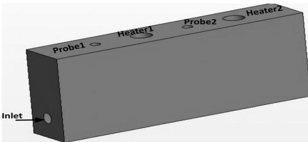
**Figure 10.** CFD Setup.
