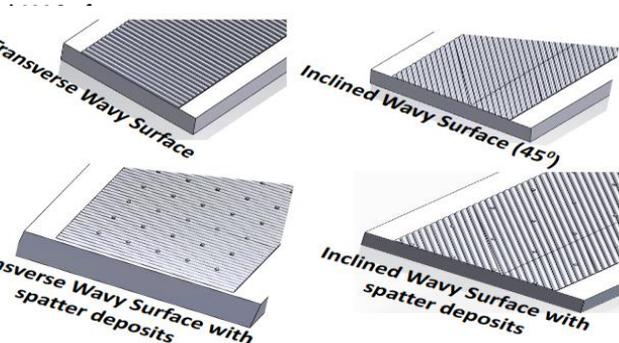
the channel were assumed to be insulated and constant heat flux was provided at the bottom of the channel. In-built laminar and turbulent flow models ( $k-\epsilon$  model) in StarCCM+ were used during the simulations.
