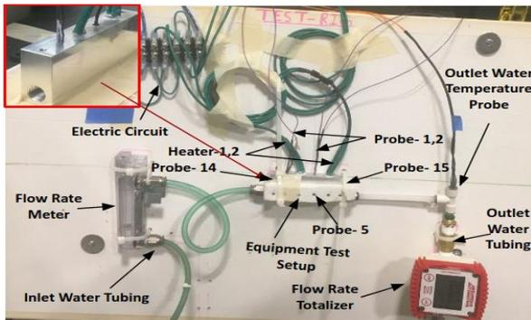
**Figure 9.** Experimental Setup.
