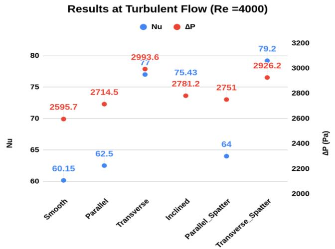
Figure 7. Nusselt Number ( $Nu$ ) and Pressure Drop ( $\Delta P$ ) for various channels for the turbulent flow case.
