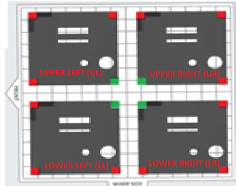
Figure 1. Benchmark's location and orientation on the build plate.
