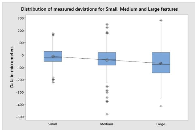
Figure 5. Measured deviation values for feature size effect analysis.
