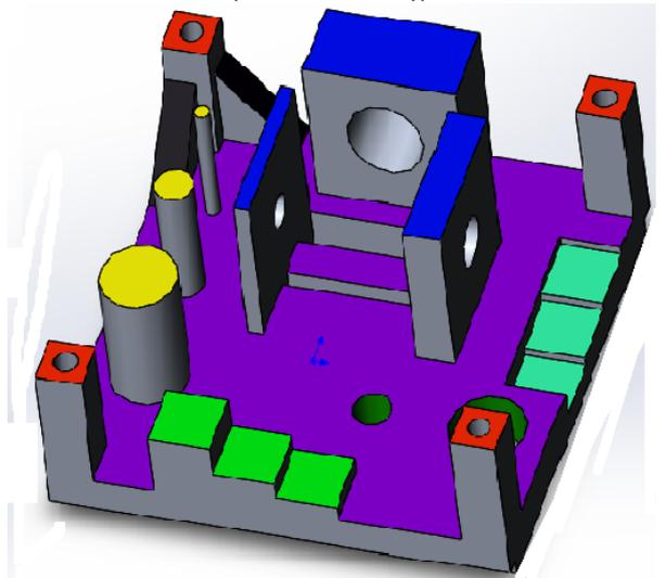
representative of the most relevant objects produced by RP processes. The geometrical features are aligned with either X or Y axis of the SLA machine to evaluate the accuracy along those axes. In addition, the sizes and locations of all features are designed to be accessible to a digital calliper's jaws. The number and types of controlled elements are as follows: linear lengths (49), diameters of holes (9) and diameters of cylinders (3).
