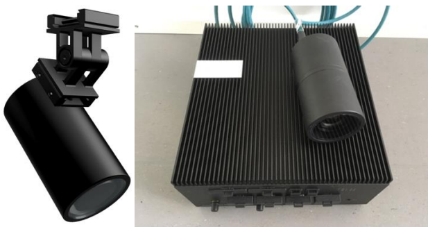
Figure 2. Vision system, comprising of an industrial camera and embedding computing system (mounting hardware not shown).
