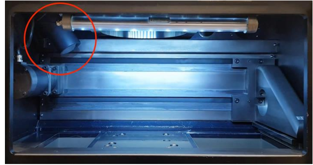
Figure 3. Vision system shown mounted in the build chamber of an EOS EOSINT M270 additive system.
