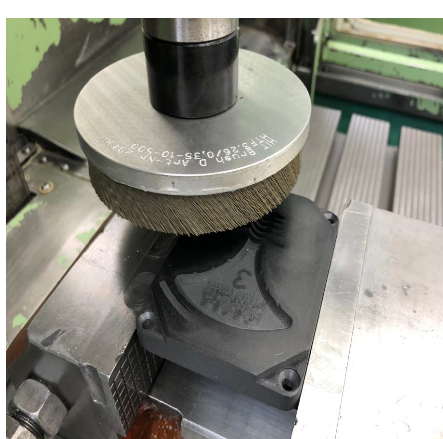
Clamped workpiece after brushing
