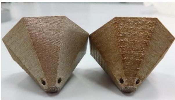
Figure 5: First sight of a downskin part with different orientation.
