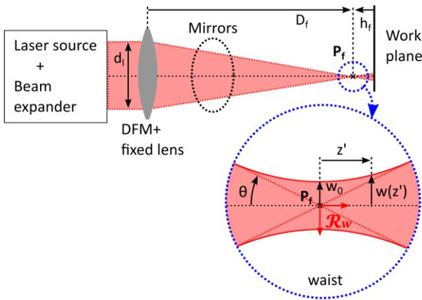
Figure 2. Parameterization and representation of the waist.
