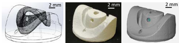
Figure 2. CAD model on the left, coated part in the center and scan model on the right.
