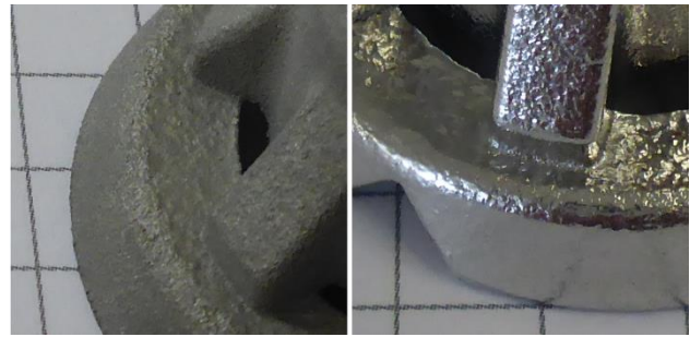
Figure 4. SLM part before (left) and after (right) PeP. PeP time 4 minutes. Grid dimensions are 5mm. Steel.
