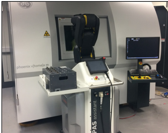
Figure 9. CT solution “v|tome|x m 300” with robotic part handling [9]
