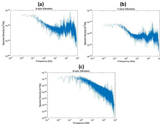
Figure 6: XCT system vibration spectral density response from (a) X-, (b) Y- and (c) Z-axes.
