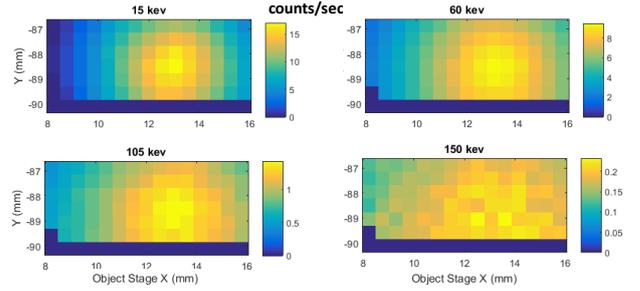
Figure 4: XCT system source map for a given energy level.
