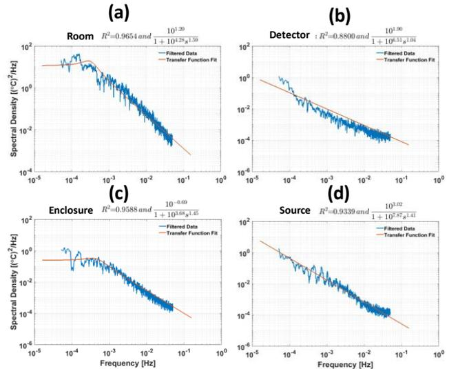
Figure 5: XCT system thermal spectral density response from (a) the room, (b) detector, (c) enclosure, and (d) source.
