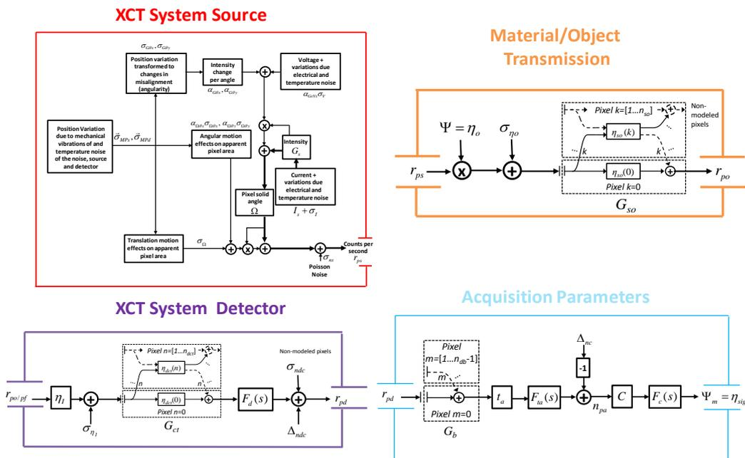
Figure 2: Signal variation flow graphs for all X-ray data acquisition components.
