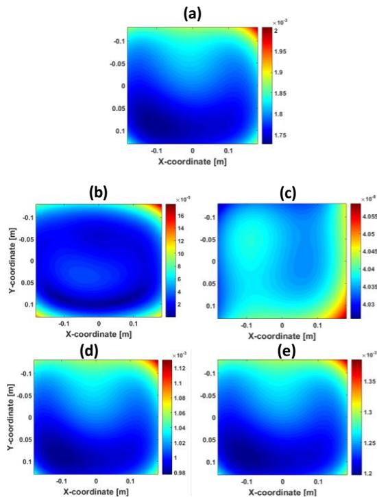
Figure 7: Uncertainty field for (a) the total noise of the XCT system, (b) mechanical vibrations, (c) temperature variations, (d) emission noise and (e) object transmission
