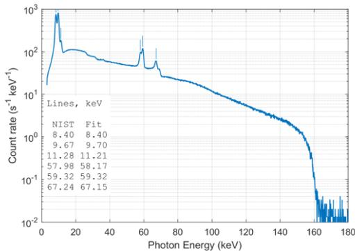
Figure 3: X-ray system spectrum for 160 kV at 0.3 W.
