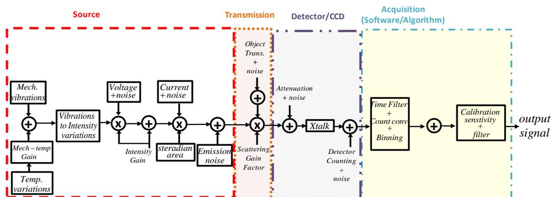
Figure 1: Graphical representation of sources of error for a conventional XCT system.
