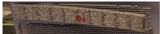
Figure 7. Directional removal of support structures for rectangular samples (as seen in Piece 2)
