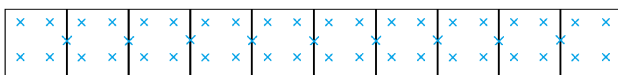
Figure 5. Points for measuring deformation before and after removal of support structures in rectangular samples (Piece 2)
