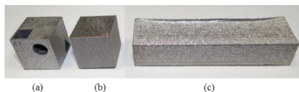
Figure 1. Pictures of the samples: (a) Al-Si-10-Mg, (b) Ti-6Al-4V LPBF cubes and (c) Ti-6Al-4V EBPF rectangular prism.
