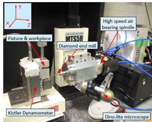
Figure 1. Experimental setup and working coordinates
