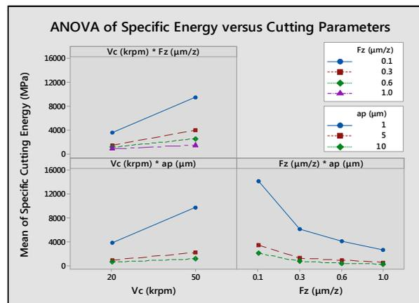
**Figure 5.** Factorial plots of specific cutting energy v.s. cutting parameters
