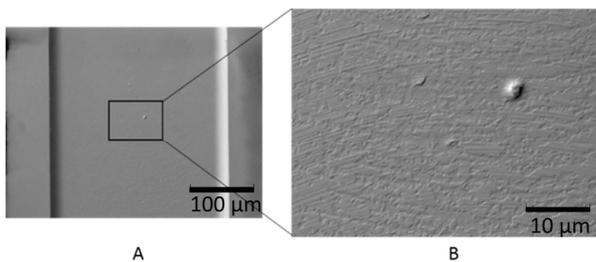
**Figure 4.** (A) Bottom of the slot machined under optimal parameters, possessing rigid edges and smooth, polishing-like surface; (B) Zoom-in view of Pic A, magnified by a total of 3 000 times, where tool marks are clearly visible, indicating that ductile mode machining was undergoing when producing this micro channel.
