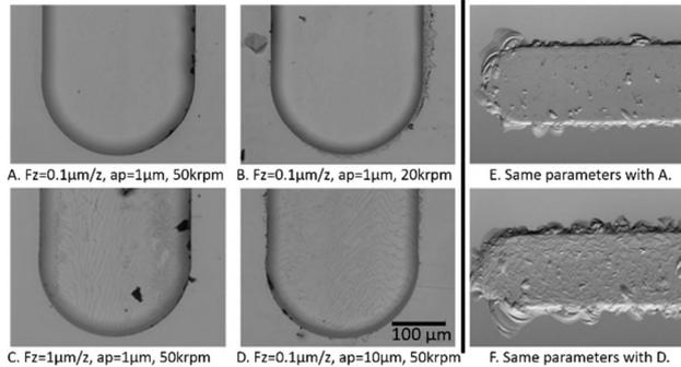
**Figure 2.** SEM pictures of micro channels. (A) Slot machined using optimized parameters; (B) Decreasing the cutting speed in A; (C) Increasing the feed rate in A; (D) Increasing the cutting depth in A; (E,F) Machining using the parameters in A and D with a UT coated tool.
